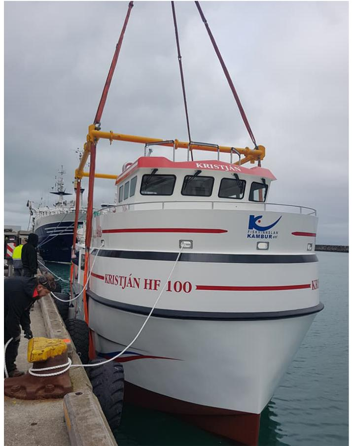
Icelandic crane rental company DS Lausnir provided lifting and rigging gear, including a frame made of Modulift beams, to lift a 45t boat into water for the first time at a harbour in Hafnarfjörður on the southwest coast of the country, about 10km south of Reykjavík.
