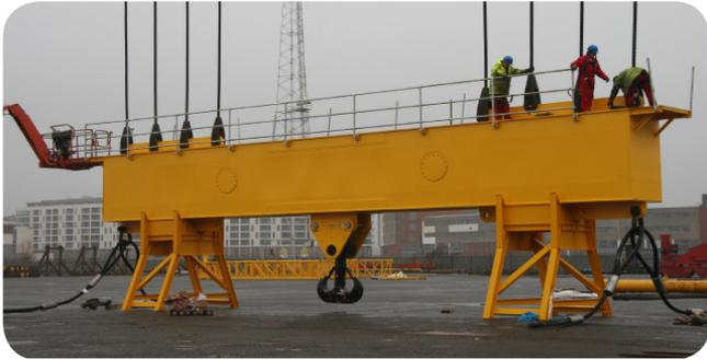
Modulift's remit was to design a rig which could not only lift the individual turbines and towers separately and assembled, but also lift three wind turbine blades in one go enabling the blades to stay in their calibrated sets for each turbine, at all times. Using the same principles of their existing standard products, Modulift succeeded in engineering a safe, lightweight, and cost-effective solution allowing Harland and Wolff to continuously store and load from January until the end of July.
