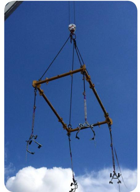
The spreader frames are also designed for lifts where there are height restrictions as the height of the rig is lower than a one-over-two solution that might be commonly
