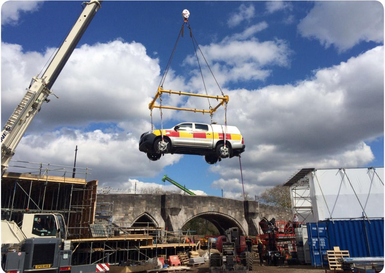
The Modulift CMOD modular spreader frame was used beneath the hook of a mobile crane as the approx. 2,000kg vehicle was lifted on two occasions during the one-day shoot. The frame combined with chain slings and clamps that attached the rig to the tyres.
